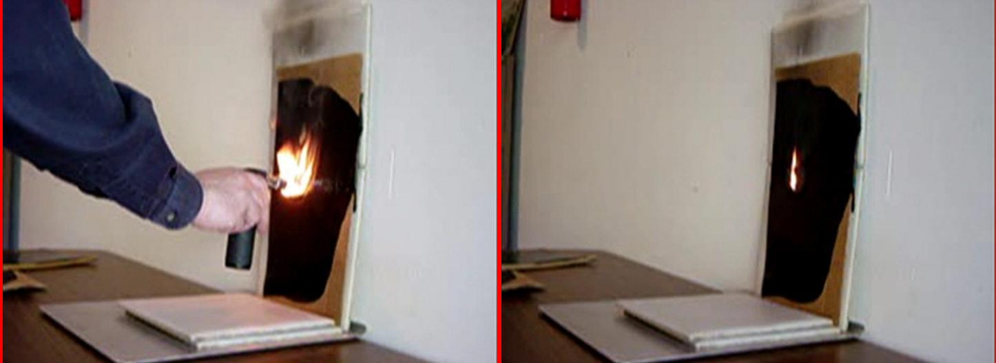
ULTRA-FLEX™ 5000 FR was ignited with a 2000°F torch for a period of 10 seconds. This test was repeated twice in the same spot within seconds of the material self extinguishing the flame.
